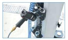
Impact wrench holder with integrated tray for support disc extensions.
