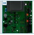
Simple visual error diagnostics thanks to LEDs mounted on the circuit board
