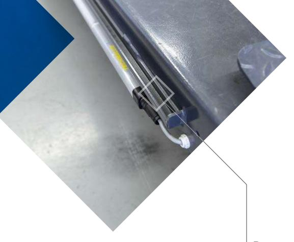
Lowering device for chassis alignment included as standard, with precision-adjustable lock ladder and electromagnetically operated latches
